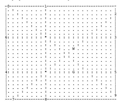
W and G indicate the airports: W for White Airport and G for Gray Airport. On the H19/H89 screen White Airport shows up as a white block, and Gray Airport as a gray block. Navaids are indicated with an "\*", and airways show up as lines of colons with entry/exit fixes on each end indicated by the digits 0-9. Note that numbers on the ends of each airway add up to 9, to make them easier to locate. The distance between adjacent dots is one mile -- horizontally, vertically, or diagonally.
